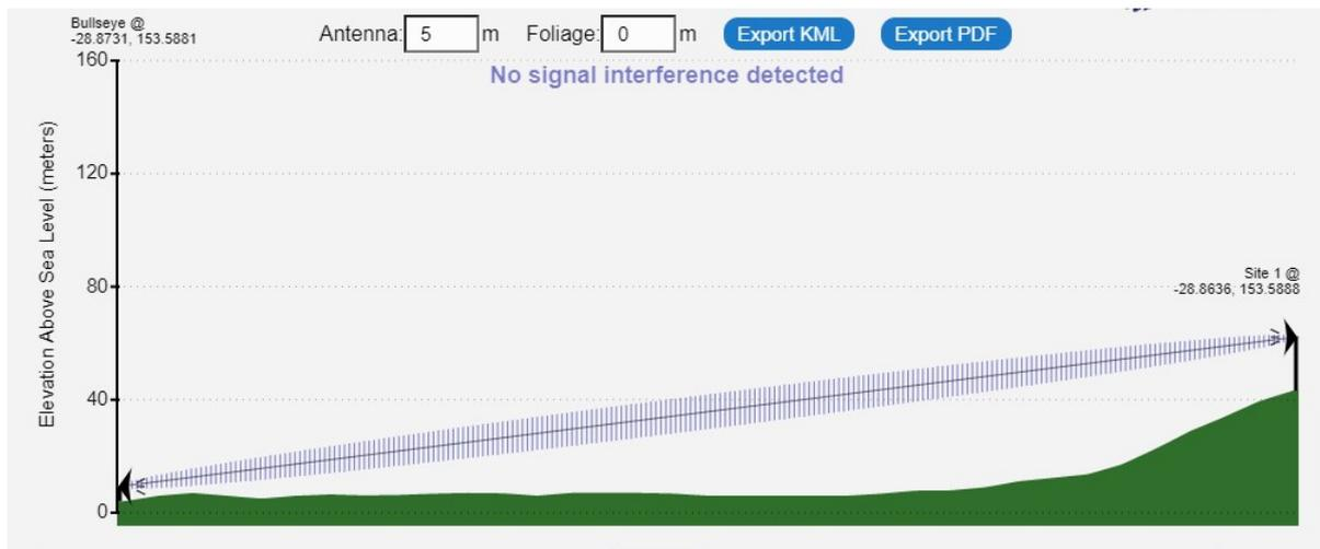
Assuming there is no non-terrain obstruction, and the predicted signal strength is close to the reality from station at *Suvla Street BALLINA*, the receiving antenna is recommended to be raised to 5 m AGL in this setup to achieve a clearer First Fresnel Zone, and then a better connection can be attained.
