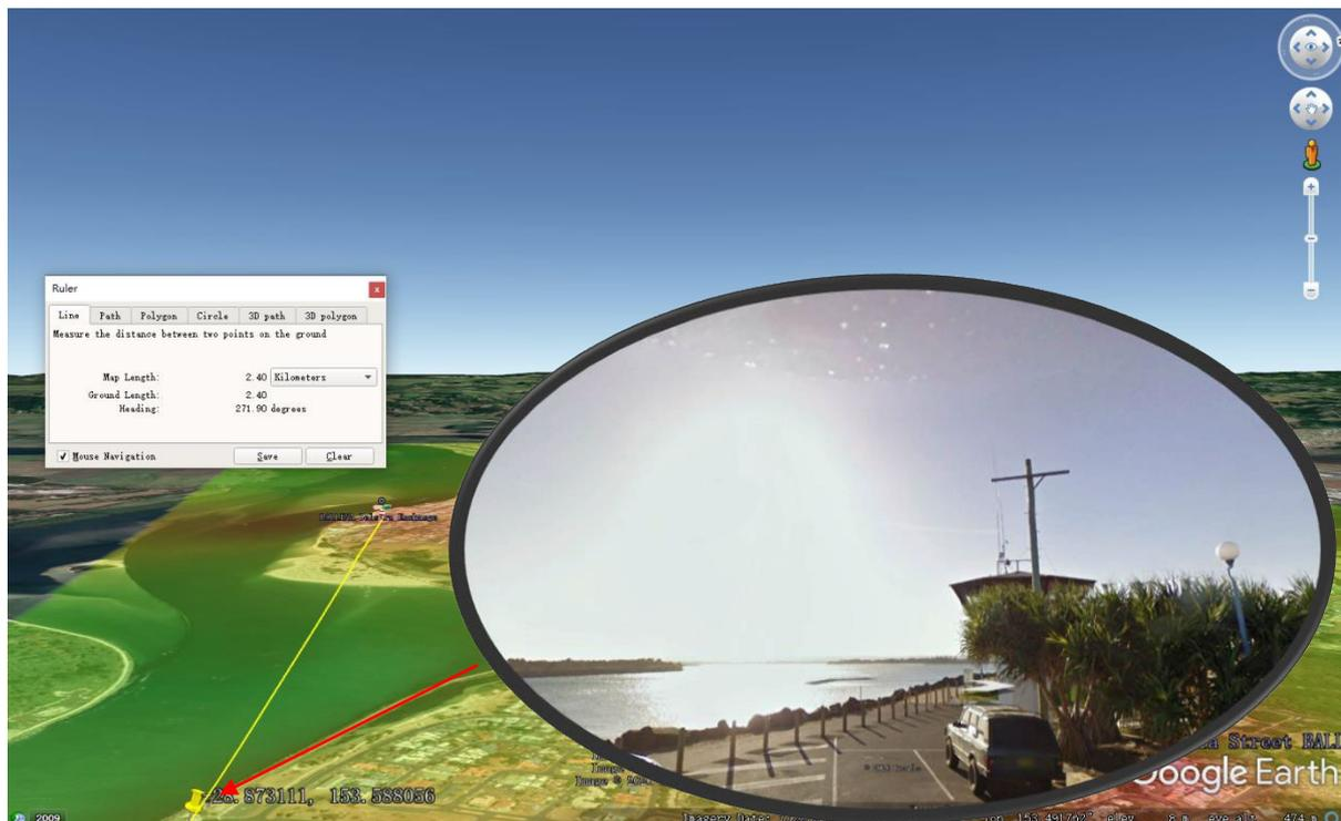
As can be seen from the image above, there are various buildings and trees between *BALLINA Telstra Exchange* and the site. As a result, they may be *a small variance* in the actual received signal strength from the estimated signal strength..
