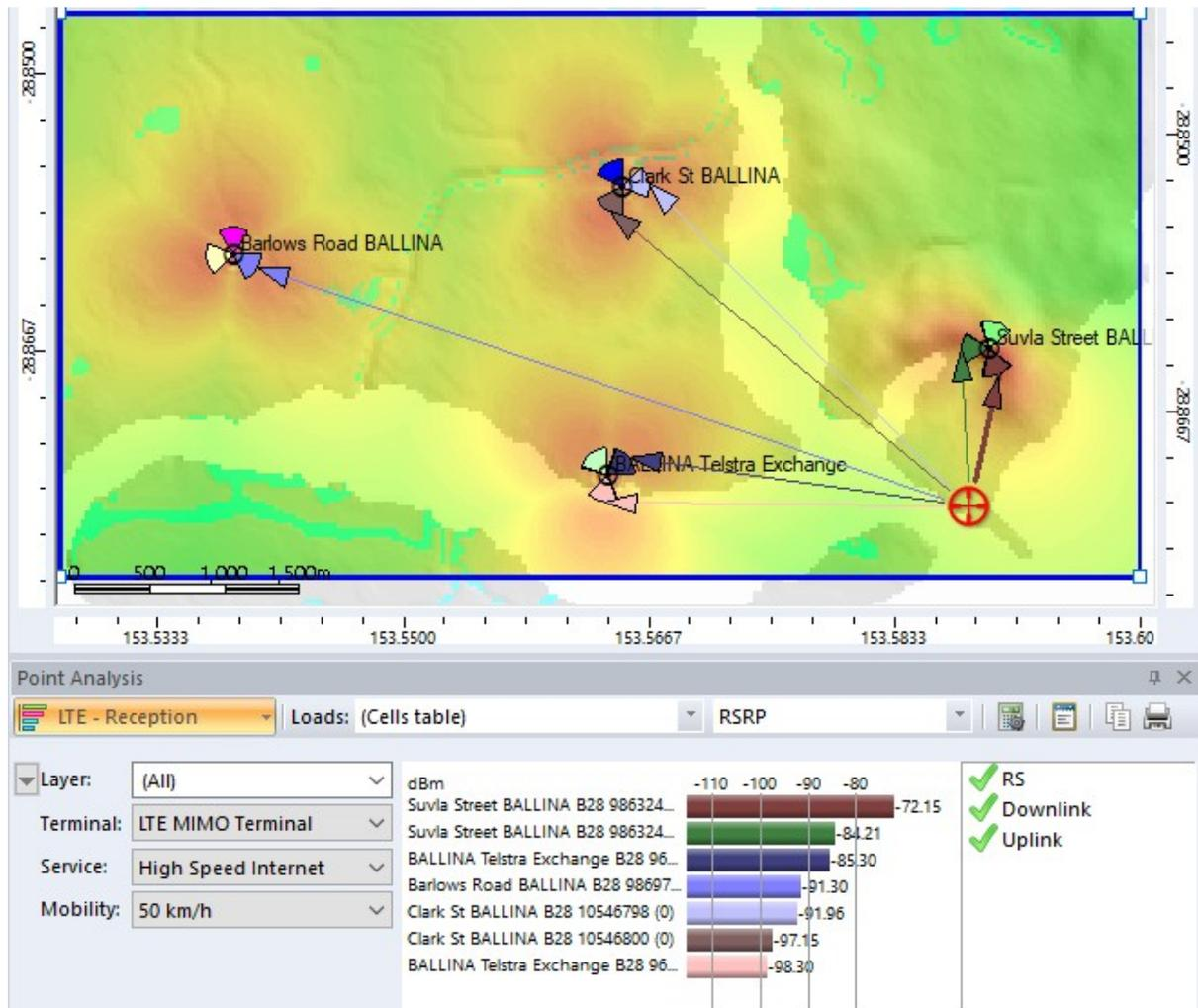
Based on the base station information from ACMA and SRTM geographic data, the image above shows the simulated heatmap of *Telstra 700MHz* signal coverage.
