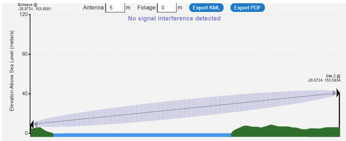
Assuming there is no non-terrain obstruction, and the predicted signal strength is close to the reality from the station at *BALLINA Telstra Exchange*, the receiving antenna is recommended to be raised to 5 m AGL in this setup to achieve a clearer First Fresnel Zone, and then a better connection can be attained.
