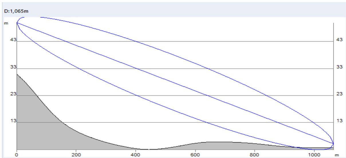
The image above shows the terrain profile from *Suvla Street BALLINA* to the site based on the SRTM digital elevation model. The distance between the two points is *almost 1.06 km*, and *both LOS and First Fresnel Zone are nearly clear*. Therefore, service reliability from it should be *high*.
